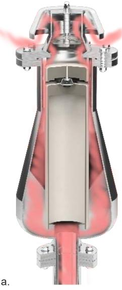
Air enters the valve and flows through the annular space between the floats and the valve body and discharges from the Large Orifice into atmosphere.
