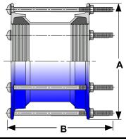
REXUS KII Couplings can be manufactured to any pipe OD from DN50 up to DN1600 as standard and Pressure Ratings PN10, PN16, PN25 and PN40 as standard.
