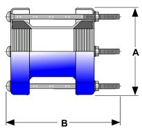
REXUS KII Couplings can be manufactured to any pipe OD from DN50 up to DN1600 as standard and Pressure Ratings PN10, PN16, PN25 and PN40 as standard.
